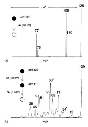
Fig. 3. (a) Low energy CA spectrum (Ar,  $20 \,\text{eV}$ ) of protonated thioanisole (m/z 125) and (b) CA spectrum ( $N_2/8 \,\text{keV}$ ) of the [M + H–CH<sub>3</sub>]<sup>•+</sup> ions generated by collision-induced methyl loss from protonated thioanisole. (#) Artefact peaks; (\*) peaks already observed without the presence of the collision gas.
