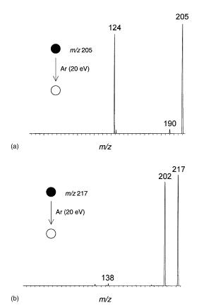
Fig. 8. CA spectra (Ar,  $20 \,\mathrm{eV}$ ) (a) of methylated 4-bromothiophenol (m/z 205,  $^{81}\mathrm{Br}$ -containing ions to avoid interferences) (fragment ion peaks amplified by a factor 15) and (b) of methylated 4-bromothioanisole (m/z 217) (fragment ion peaks amplified by a factor 5).
