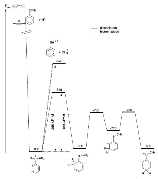
Fig. 4. Potential energy surface, obtained at the B3LYP/6-311++G(d,p)+ZPE level of theory, of the  $C_7H_9S^+$  isomers of protonated thioanisole. The transition states corresponding to proton migrations are shown.
