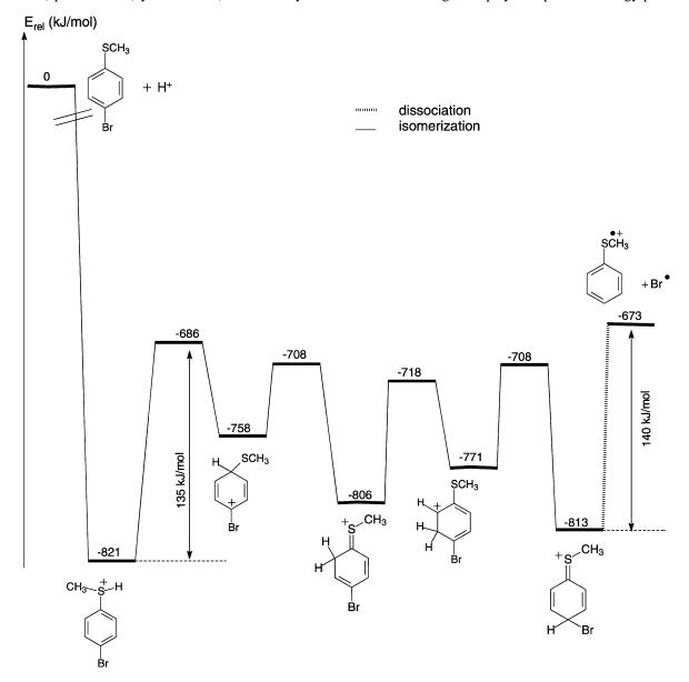
Fig. 6. Potential energy surface, obtained at the B3LYP/6-311++G(d,p)+ZPE level of theory, of the  $C_7H_8BrS^+$  isomers of protonated 4-bromothioanisole. The transition states corresponding to proton migrations are shown.
