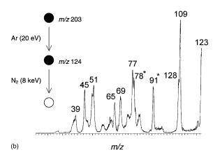
Fig. 5. CA ( $N_2/8 \,\text{keV}$ ) spectra of the molecular ions of thioanisole (m/z 124) (a) and of the [M+H-Br] $^{\bullet+}$  ions generated by collision-induced bromine loss from protonated 4-bromothioanisole (b). Asterisk indicates the peaks observed without the presence of the collision gas.
