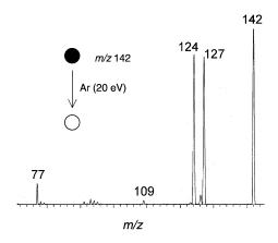
Fig. 7. CA spectrum (Ar,  $20 \,\text{eV}$ ) of thioanisole methylated by CD<sub>3</sub>I in the CI source (m/z 142). The intensities of the signals corresponding to the collision-induced fragments are amplified by a factor 30.
